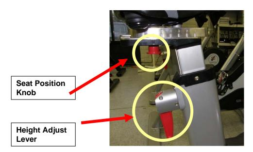
2.1 Remove the seat assembly completely from the seat post by fully pulling down on the red seat position knob.
