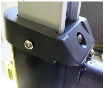
5.4 Tighten the three collar screws snugly, but do not overtighten.
