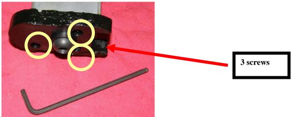
2.6 Remove the three screws holding the bracket on the seat post using the 2.5mm Allen wrench. Discard bracket but set aside screws for re-use
