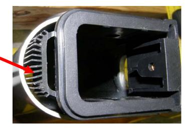
3.2 Fit the outer collar piece on to the seat post and inner piece. Inspect and verify that the two holes in the collar line up with the holes in the frame. The collar holes may be opened up slightly as needed to ensure that the screws can be installed properly.
