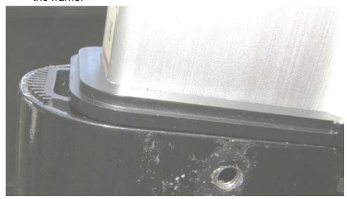
5.3 Slide the outer collar piece into place over the inner piece and the frame. Loosely install the two side screws and the rear screw and verify smooth operation of the seat post.
